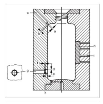
Figure 35: Suitable Methods for Mould Cavity Venting
