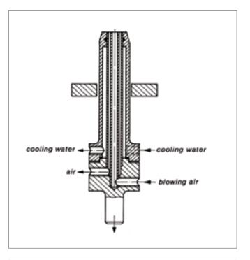
Figure 29: Section Through a Blowing Mandrel for Compressed Air Cooling
