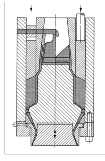
Figure 19: Tubular Plunger Accumulator (more recent design) (design: Kautex-Werke, Hangelar)
