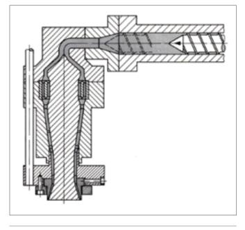
Figure 13: Reciprocating Screw Accumulator
