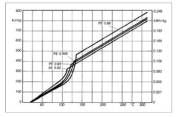
Figure 3: Enthalpy of Various Polyethylenes as a Function of Temperature
