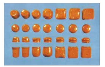
Figure 59: Blowing Investigation (coffee container with lid)
