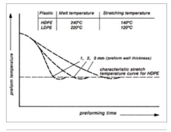
Figure 57: Temperature Curves for Injection Moulded Pre-forms Based on Optimum Stretching Temperatures for Polyethylene
