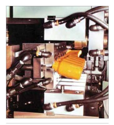
Figure 50: Mould Arrangement in Injection Blow Moulding
