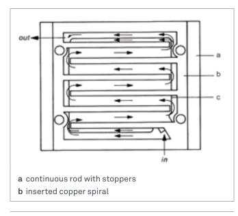
Figure 25: Cooling Channels with Labyrinth-type Water Flow
