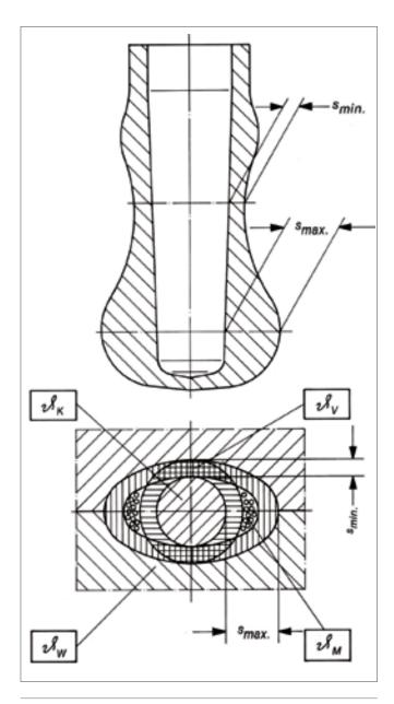
Figure 53: Wall Thickness Relationships on the Pre-form
