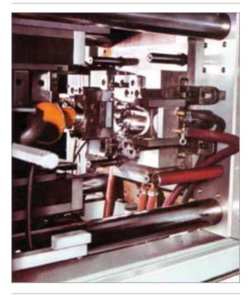
Figure 51: Injection Blow Mould Machine
