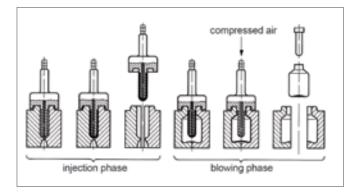
Figure 49a: Basic Principles of Injection Blow Moulding
