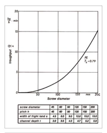
Figure 4: Specific Throughput Q/n as a Function of Screw Diameter
