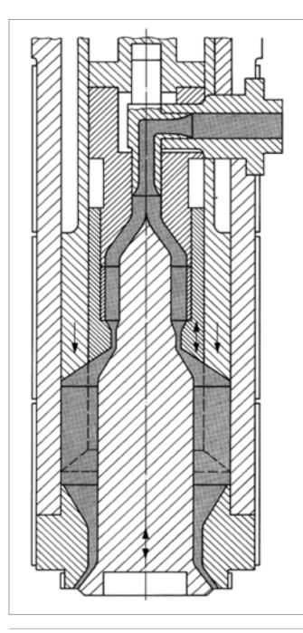
Figure 21: Tubular Plunger Accumulator (design: J.M. Voith, Heidenheim)
