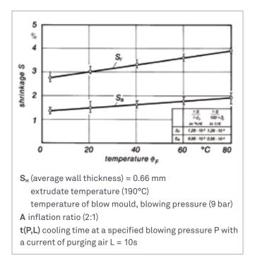
Figure 37a: Axial and Radial Shrinkage of an Axially Symmetrical High Shouldered HDPE Bottle as a Function of Mould Cavity Temperature (measured after 14 days storage at room temperature)
