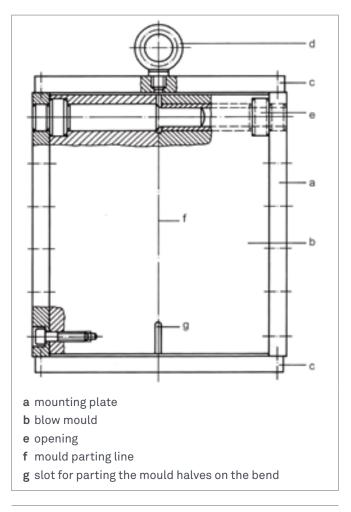
**Figure 23:** Mould Block with Transverse Bars (C) and Eyebolt (D) for Mounting
