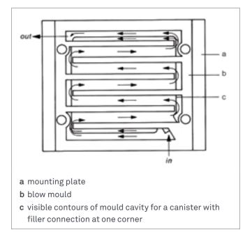
Figure 26: Channel System with Labyrinth-type Water Flow Produced by Baffles
