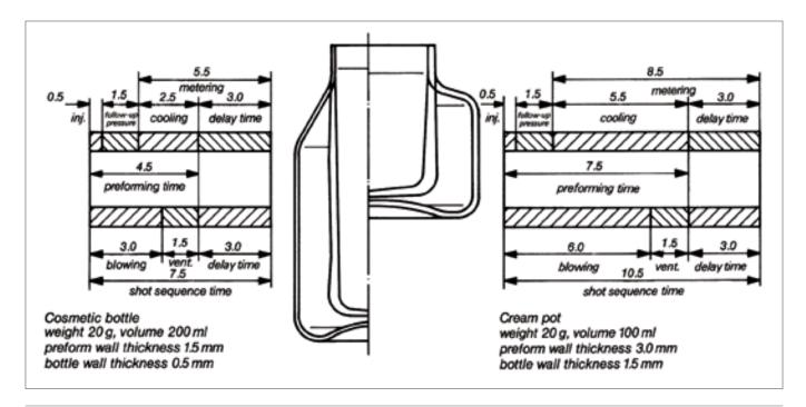
Figure 60: Shot Sequence Time as a Function of Pre-form Wall Thickness at Constant Article Weight
