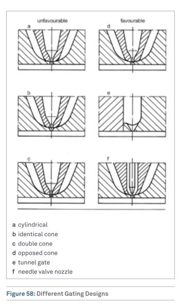
It should be noted, too, that follow-up pressure is used in the injection moulding stage of injection blow-moulding. The amount of pressure and hold-on time depends on the size of the gating and the type of plastic.
