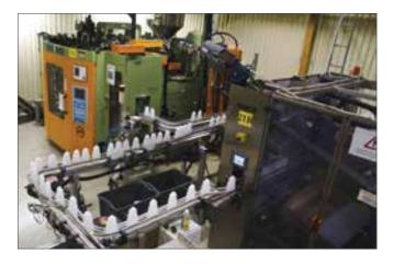
Figure 5: Dual Parison Blow Moulding Machine
