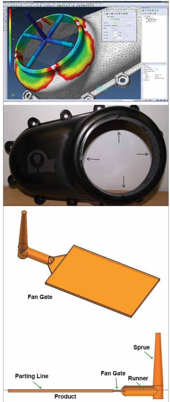
Figure 20: Photos Illustrating Multiple Pin Gating and Fan Gating
