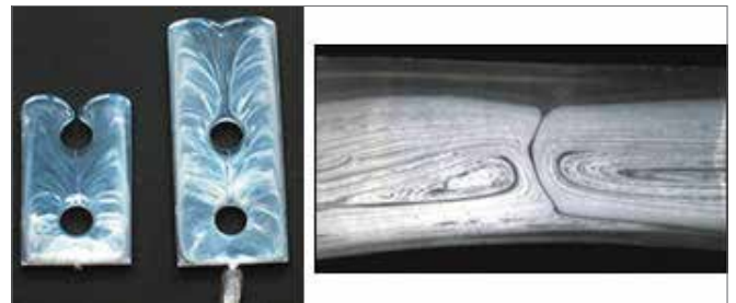
Figure 21: Mouldings Illustrating the Formation of Weld Lines When Two Melt Fronts Meet
