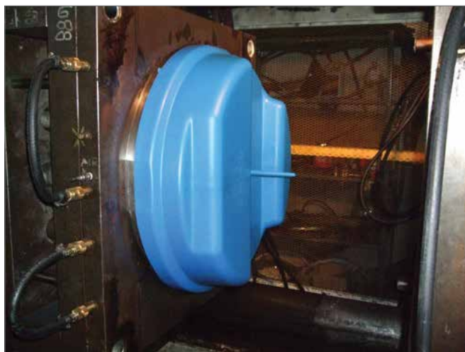
Figure 2: Finished Moulded Part including Sprue Injection Point
