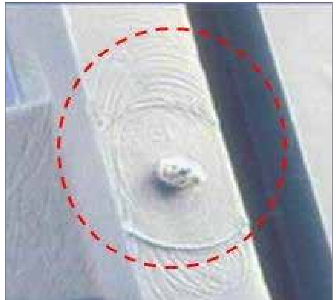
Figure 12: Photo Illustrating 'Chevron' Rings on an Injection Moulded Surface
