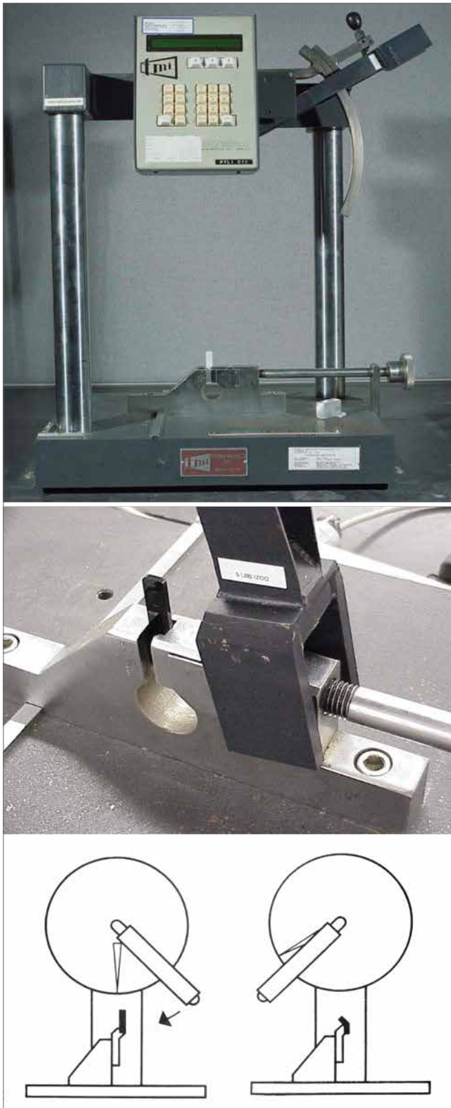
Figure 15: Impact Machine Showing Sample Holder and Process of Use
