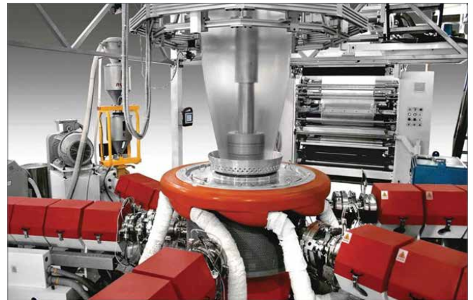
Figure 3: A Modern Blown Film Coextrusion Line with 5 Extruders
